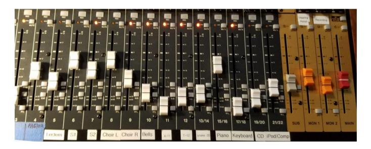
The vertical column for each channel has controls all the way from the top to the bottom of the board. The very top of the channel has input sources, which can be XLR (the round back plug with three pins) or a quarter inch jack (smaller round silver hole). We'll cover the middle knobs later on, but for now, let's move down to the white sliders, which are volume control for that channel, and then the three square buttons at the bottom (MAIN, SUB and PFL), that control where the output goes.
