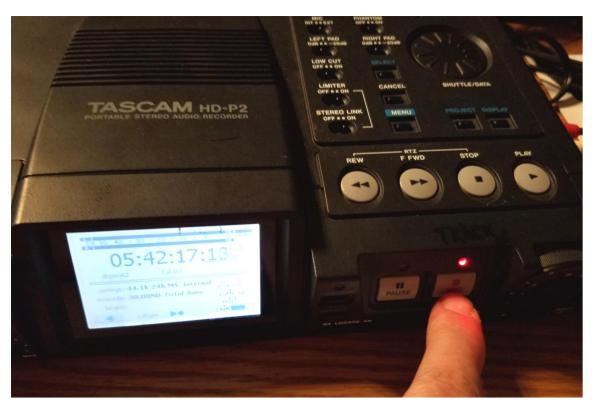
36. To end the recording, push the round STOP button on top.
