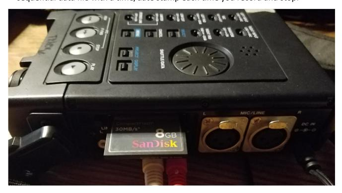
38. To shut down the recorder, toggle the POWER button again. You will be prompted on the screen to Confirm the shutdown. Push the Select button on top of the unit to Confirm the shutdown.
