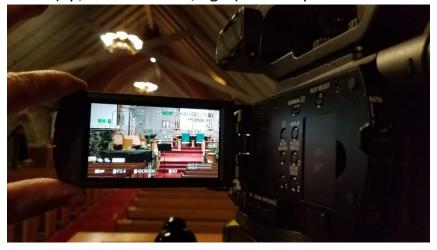
13. The ring behind the lens is used to Zoom and Focus. There is a slider switch right next to the ring. Push it up to Zoom, or down to Focus (it will autofocus). Move the camera and zoom slowly, or it is very disorienting for the viewer. There is also a button on the right top side of the camera that zooms in/out that is easier to access.
