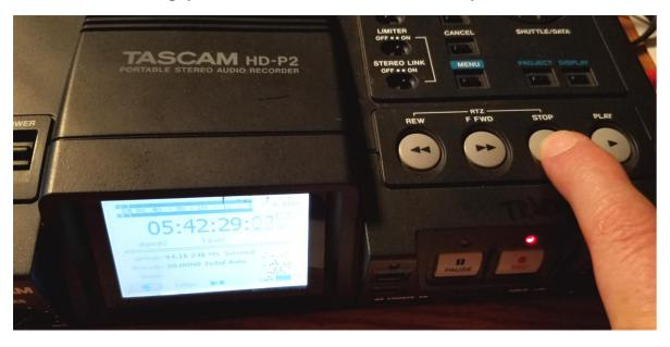
37. The audio files save to a compact flash drive that plugs in the right side or the recorder. Just leave it there until Deb comes and takes it out to edit the file and put the audio on the website. We record the entire worship service. The recorder will make a new sequential data file with a time/date stamp each time you record and stop.
