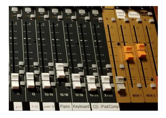
30. Channel 13/14 is labeled Snake 20 because it's connected to the Snake cable (up front under the right side choir pew). In Snake 20, there is a quarter inch cable that can be used for guitar. The piano and choir mics are also run through the snake cable. The snake is really just a set of inputs and outputs that run from the stage to the soundboard.
